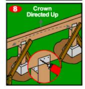
8. Measure and cut to length girders to length. Eyeball each girder to determine which way it crowns. Place each girder in position on top of the posts with the crown of the girder directed upwards. Screw the girders into place through the post cap brackets with screws and a screw gun.
